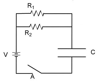
(a) What is the effective resistance of the combination of resistors  $R_1$  and  $R_2$ ? [4 points]
