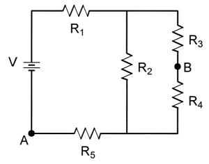
(a) Solve to determine the total current drawn from the battery. [6 points]
