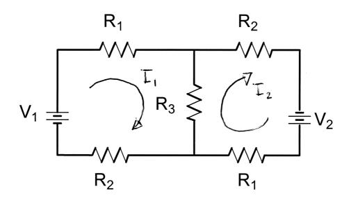
(b) Using the current directions that you assumed in part (a) carefully write down the two equations describing the potential around each loop. [10 points]
