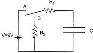
(a) At what time after the switch is connected to A will the voltage across the capacitor be 5.6 V? [4 points]
