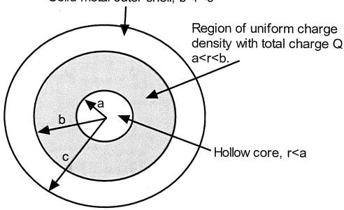
(a) Derive an expression for the charge density  $\rho$  in the region of uniform charge given that the total charge in the whole shell is Q. [3 points]
