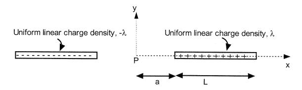
(a) For this part of the problem consider only the positive line of charge to the right of the origin. Determine an expression for the E-field the positive line charge produces at the origin P. What is the direction of the E-field vector? [8 points]
