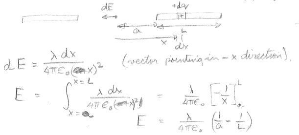
(b) Determine an expression for the total E field produced by both line charges. (Hint: you should be able to use your result from part (a)). [3 points]
